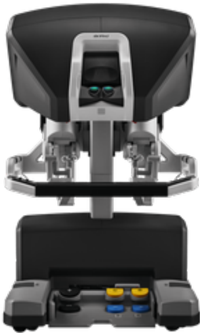
Figure 3. dVSS Surgeon Console
