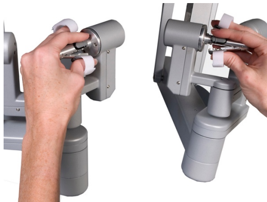
Figure 10. dVSS control grips
