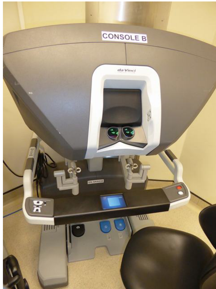
Figure 9. dVSS surgeon console
