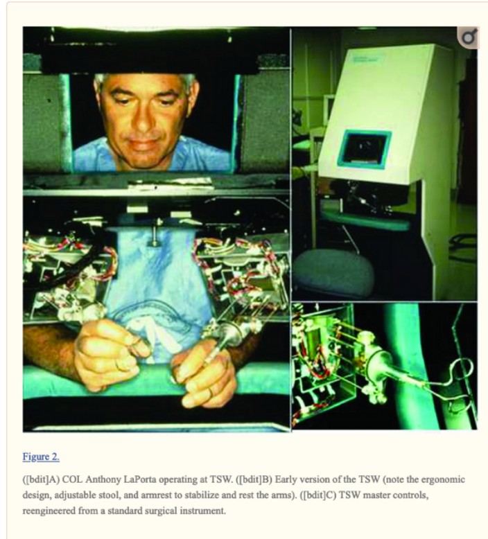
Figure 11. Telepresence surgeon's workstation (TSW)
