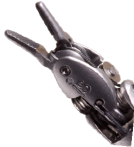
Figure 6. Large needle driver
